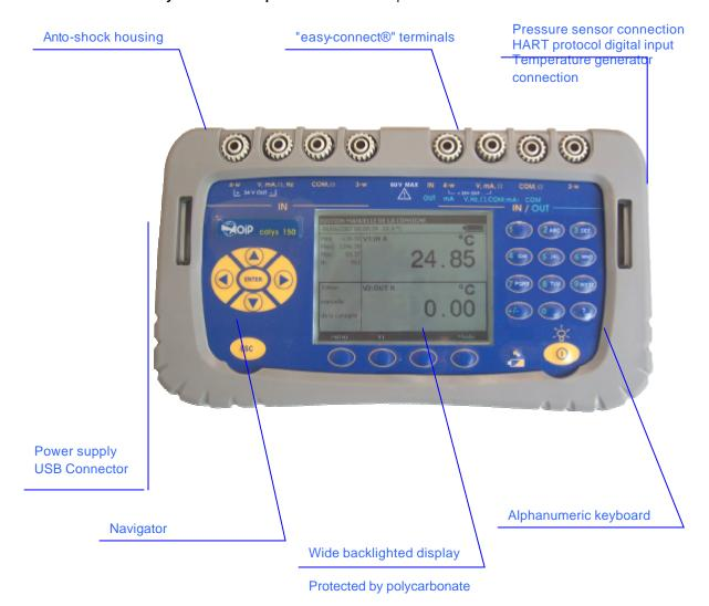
Calys 150 is delivered in standard with a strap and a stand for desktop use, a quick battery charger, and a set of 6 measuring cables with crocodile clips
